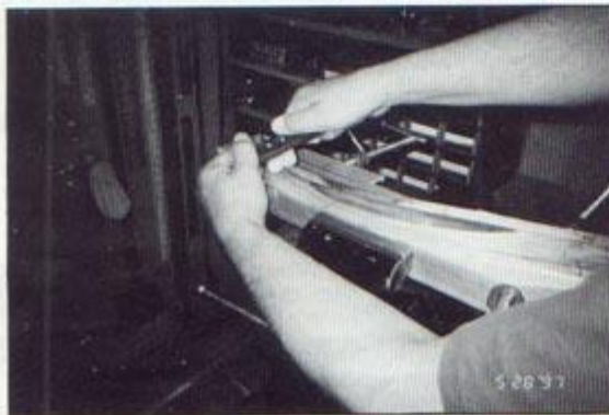
The fairing is clamped in the jig and the roller tool starts the bend.
