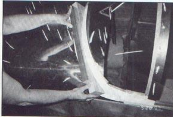
The 2x6 clamping jig follows the contour of the windscreen
