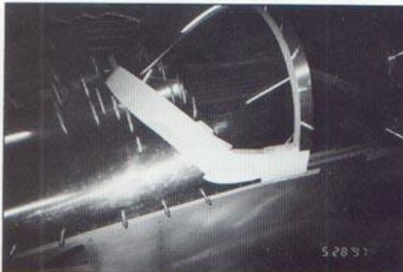
A posterboard template is fit to the windscreen. The bottom edge follows the line projected on the top skin.
